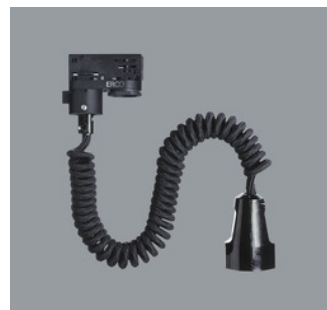
79052.000 ERCO 3-circuit adapter with earthed coupler. 250V, 6A. Spiral cable 3x0,75mm². L 700/1400mm. Black
