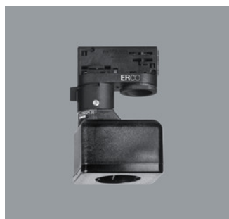
79024.000 ERCO 3-circuit adapter with earthed socket outlet. 250V, 10A. Polymer. Cover: Polymer, black. L 71mm, B 56mm, H 90mm. Black CE
