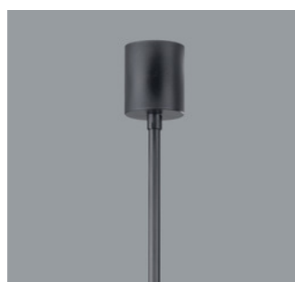
12445.000 Pendant tube suspension Pendant tube: metal, powder-coated. ø 13mm, L 1,040mm. Baldachin: polymer. ø 64mm, H 73mm. Load: 20kg. Black CE Only in conjunction with 78670.000 79550.000 79555.000 79560.000 79565.000 79570.000
