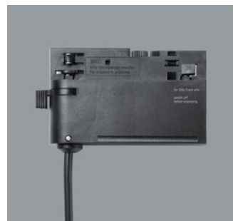
79048.000 ERCO DALI adapter for 250V, 1A pendant luminaire, with strain relief. Polymer. Connection cable 5x0,75mm 2 , L 1500mm. Requirements placed on DALI control gear: DALI input suitable for mains voltage, max. capacity 750pF. Not suitable for DALI singlet. Black Weight 0.39kg CE
