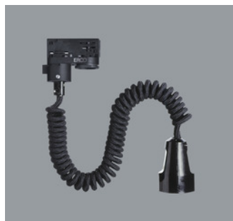
79052.000 ERCO 3-circuit adapter with earthed coupler. 250V, 6A. Spiral cable 3x0,75mm 2 . L 700/1400mm. Black
